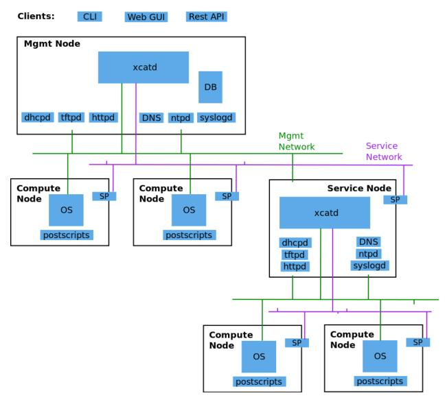
**xCAT Management Node (xCAT Mgmt Node):** The server where xCAT software is installed and used as the single point to perform system management over the entire cluster. On this node, a database is configured to store the xCAT node definitions. Network services (dhcp, tftp, http, etc) are enabled to respond in Operating system deployment.
